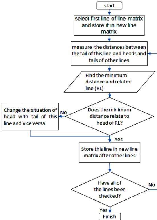
Fig. 6 Arranging and sorting algorithm
