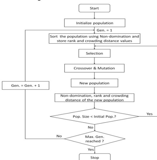
Fig. 2 Flowchart of NSGA-II algorithm
