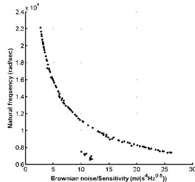
Fig. 5 Pareto optimal fronts for Brownian noise / sensitivity and natural frequency
