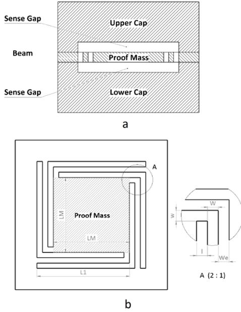
Fig. 1 Proposed micro-accelerometer a) the whole system b) proof mass dimensions
