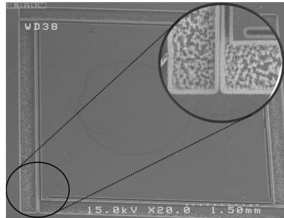
Fig. 8 SEM picture of fabricated MEMS element
