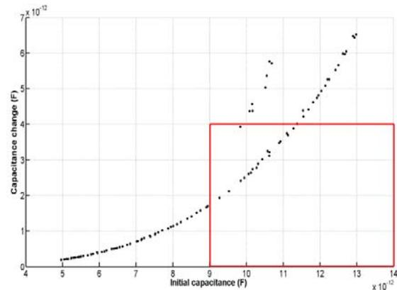
Fig. 7 Pareto optimal fronts for initial capacitance and capacitance change considering read out circuit limit (rectangular area)
