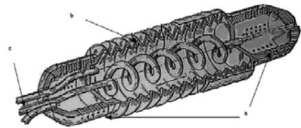
Fig.13. Pneumatic lay-out of the microrobot: (a) cylindrical clamber with suction holes and hemispherical tips; (b) rubber bellow; (c) service pipes[13].
