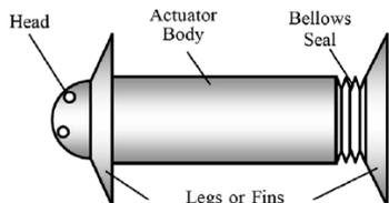
Fig. 4. Schematic structure of the Lu et al. inchworm robot[4].
