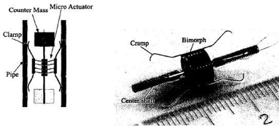
Fig. 11. Developed locomotive mechanism using multi-layered PZT Bimorph actuator.
