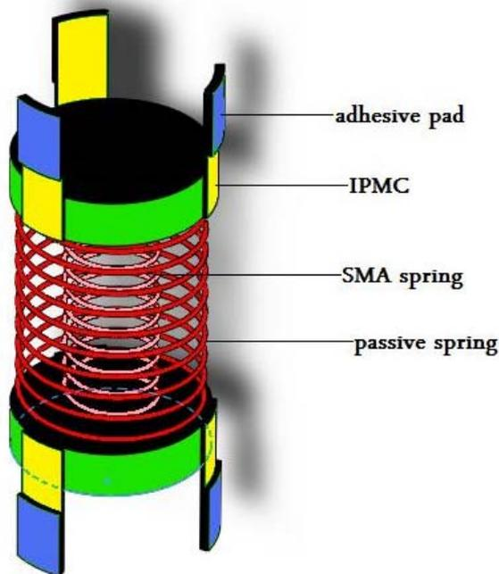
Fig. 23. Schematic diagram of the designed microrobot
