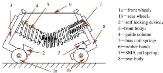
Fig. 16. Schematic diagram of the micro-wheeled-robot[16].
