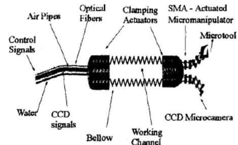
Fig. 14. Scheme of Dario et al. microrobot[14].
