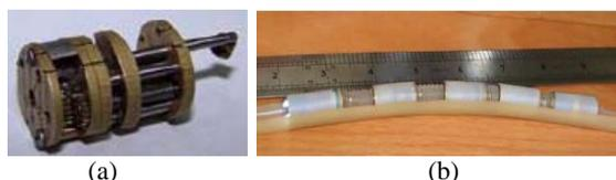
Fig. 5. (a) A driving segment and (b) Microrobot as a whole[5].
