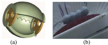
Fig. 18. (a) Earthworm module, (b) The artificial earthworm[18].
