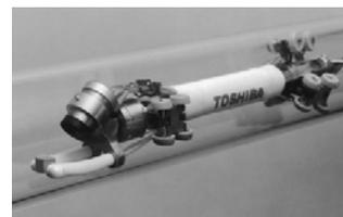
Fig. 8. Micro inspection robot carrying a recovered object in a 1-in pipe[8].
