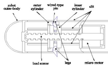
Fig. 6. Concept design of microrobot[6].
