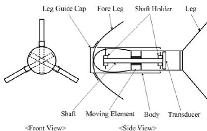
Fig. 12. Conceptual design of the proposed locomotive mechanism in Hyunjun park et al. [12].
