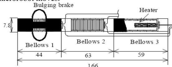
Fig. 9. Schematic view of Kato et al. microrobot[9].
