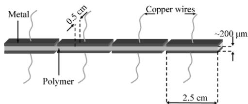
Fig. 3. Schematic IPMC worm presented by Kim et al.[1].
