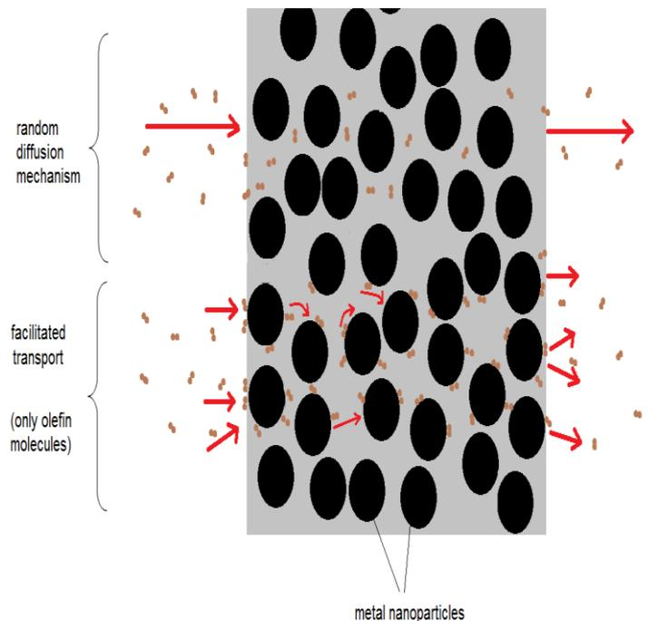
Figure1: Diffusion mechanisms in nanocomposite membrane
