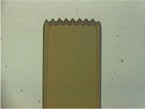
Fig 1: Shipley 1813 developed by MIB developer
