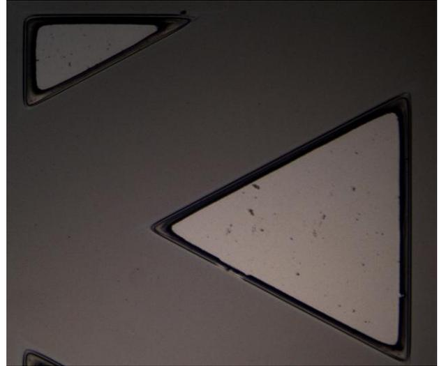
Fig 3: KMPR sample developed by commercial solution
