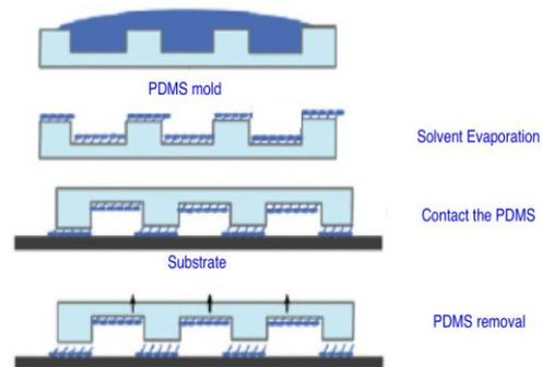
Fig1. Soft lithography- Left: Capillary molding, Right: Contact printing [4]
