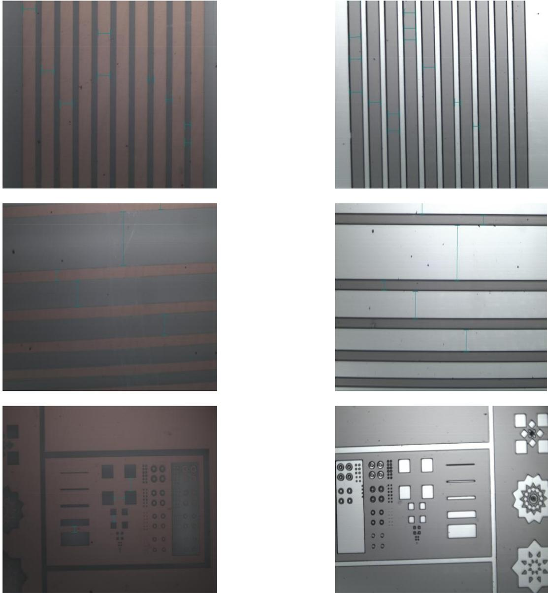
Fig3. Optical Microscope images- Left: image on Chrome mask, Right: image on silicon wafer
