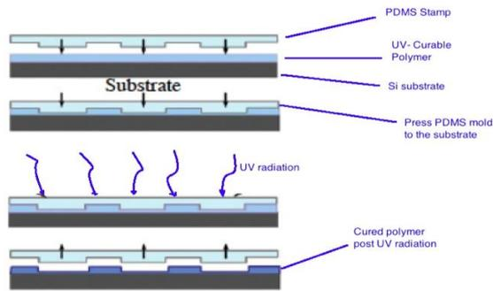
In this paper, images of a binary mask transferred to a silicon wafer using contact photolithography. Imaged silicon wafer was then used for soft lithography method to form PDMS stamp.
