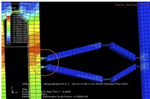
Figure2 Image of ABAQUS full body model analyze of microgripper. As shown the maximum stress occurred in design is much lower than yield stress. The critical joints determined with a circle.
